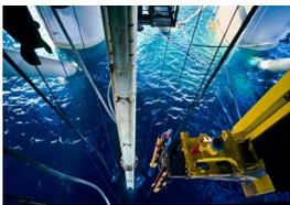
As water depths have increased, steel riser design solutions have been extrapolated from successful shallower water applications. Whilst there has been some investigation and application of other materials such as aluminium and titanium, steel has remained technically and commercially the material of choice.
